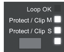
Loop(s) faulty, input too high or driver overloaded
